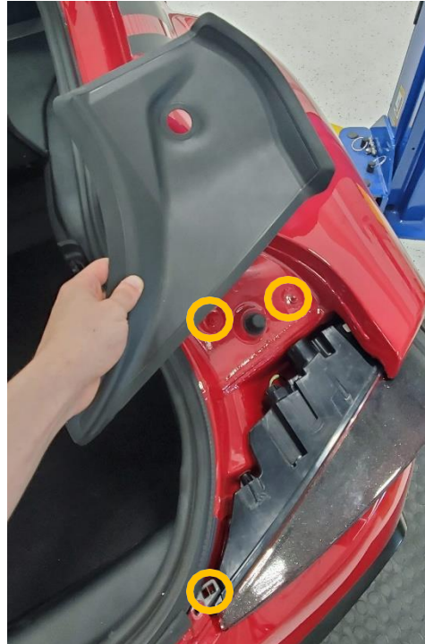
Removed cover, showing clip locations
