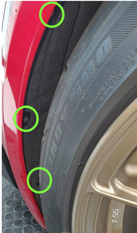
Rear wheel well liner bolt locations (3)
