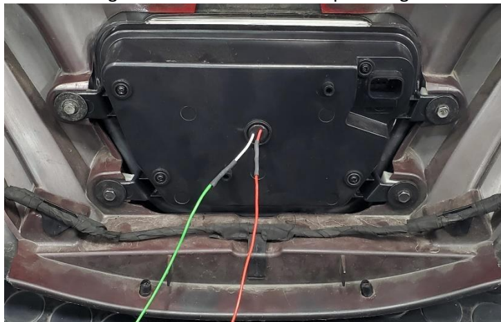
OLM 4 th brake light installed into bumper
