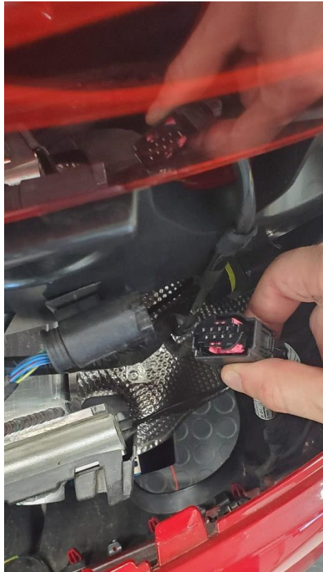
Disconnected rear parking sensor connector
