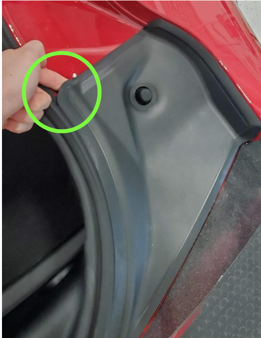
Installed cover, showing pry point
