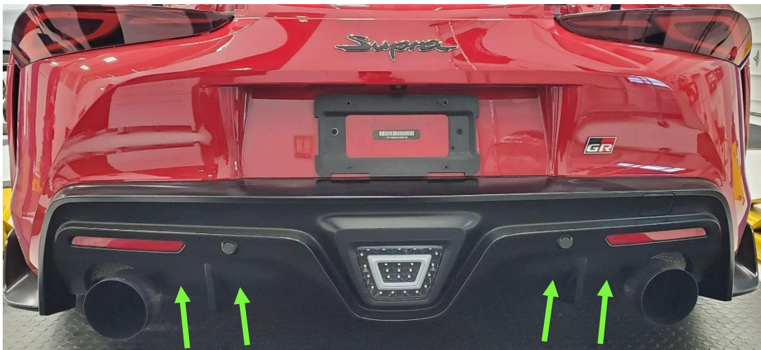
Diffuser bolt locations (4)
